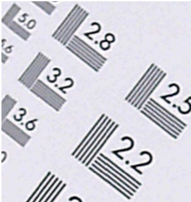
Around each character is a white halo. The halo is the result of a very heavy sharpening to boost the clarity of the B/W transition. In Color or G/S scanning a very low filter is most effective. However, for B&W scanning the background is washed out and only the black is left so a heavier filter can improve the quality of a cheaper scanner.
