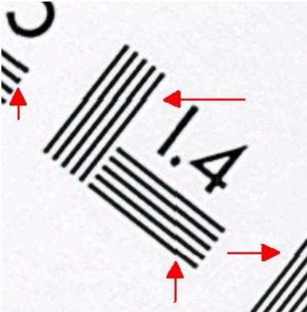
My guess here is that the image was de-skewed using a very simple shift both horizontal & vertical. This is not the technique used on better equipment.
